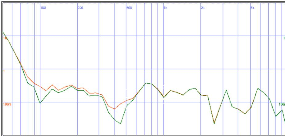
THD (red) and 3<sup>rd</sup> Harmonic (green) at a 94 dB SPL drive level (averaged from 200 Hz to 2 kHz).
